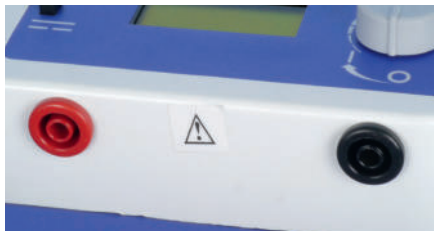
(3) Sockets to connect cables to electrodes
